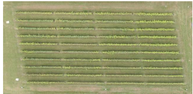
Figure 1: Grapevine test field consisting of 240 test plots. Also visible are the large radiometric targets (left) and the smaller geometric ground control points (bottom).
