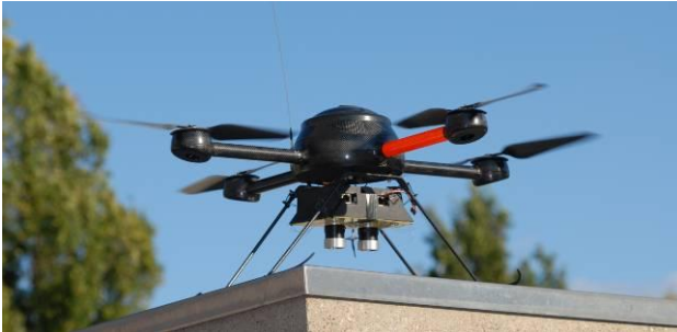
Figure 5: Quadcopter micro UAV 'microdrones md4-200' with the prototype MSMS multispectral sensor.
